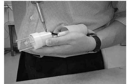
5 Insert bare wires into their corresponding color-coded terminals. Make certain there is not wire insulation under any terminal clamp. Tighten the screw clamps to 14-20 inch-pounds torque.
