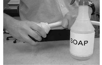
2 Push cord through the inverted end about 12 in. A tug in the opposite direction returns boot to its original shape.
