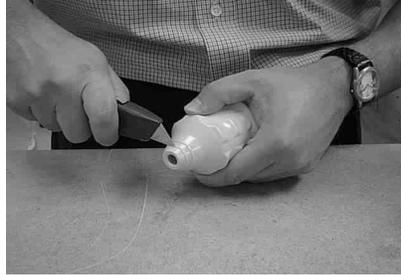
1 Cut boot at first line. Invert tapered end of the boot and apply soap solution.
